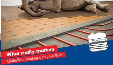
When laying laminate and wood flooring over underfloor heating, observing the thermal insulation resistance is essential. In this case, a value of 0.15 m<sup>2</sup>K/W must not be exceeded for the entire flooring installation (Underlayment + laminate/parquet).
